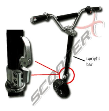
Before riding your scooter it is a good idea to check all nuts and bolts to make sure they are fastened securely. Also check your tire pressure. Should be inflated 35 PSI. Its almost time to ride!!! continue on to page 4.
