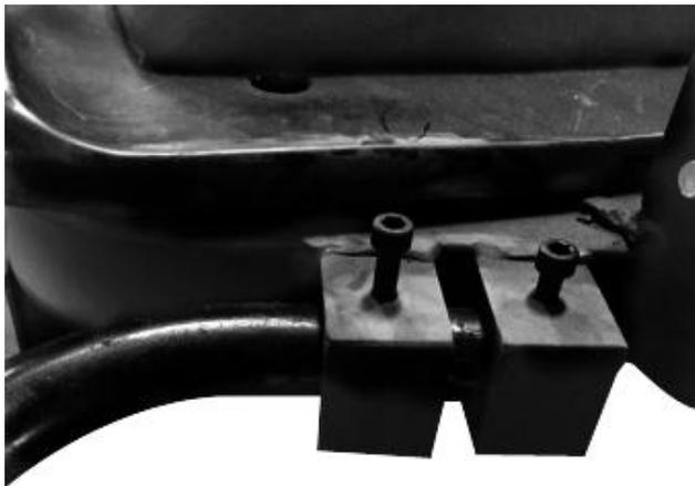
**We need to use two screws to fixed Left and right pedal**
