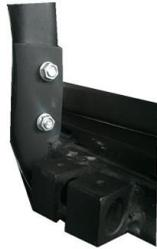
3. Remove the bolts and nuts from the connecting tube clamp. Place the connecting tube into the top opening. After aligning the hole, place the two bolts through the connecting tube and neck assembly. Twist the bolts, do not hammer them through. Tighten these two bolts with the nuts provided.
