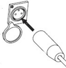
**1** Turn **OFF** power switch before charging. Plug charger into the charger port on the electric motor bike.
