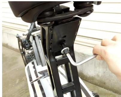
7. Attach the seat to the upper seat post and tighten the seat bolts as shown.
