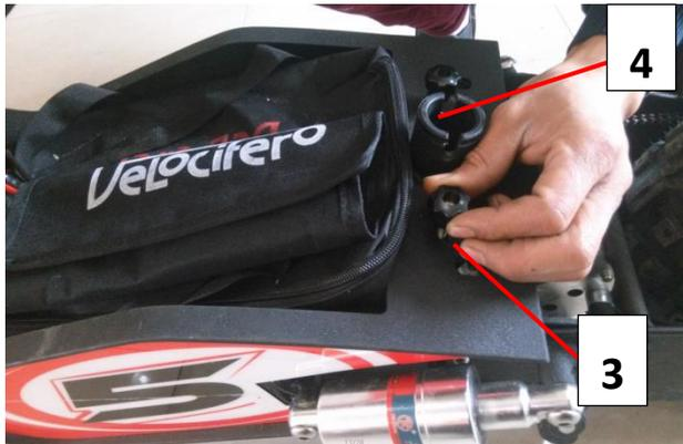
Then install the seat cushion on the sleeve as shown in figure 4. The base hole passes through the retaining bolt as shown below.
