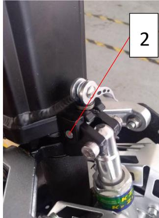
Then, use the removed bolt to go through the steering column and upper plate of the column, add the gasket and the spring pad, then tighten the nut, as shown in the figure below.
