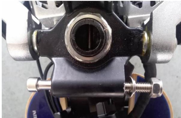
First remove the bolts and nuts and place the steering column upright on the upper plate of the column.
